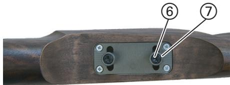
3. Loosen the relevant screw (6) of the inside the guide bolt (7).
